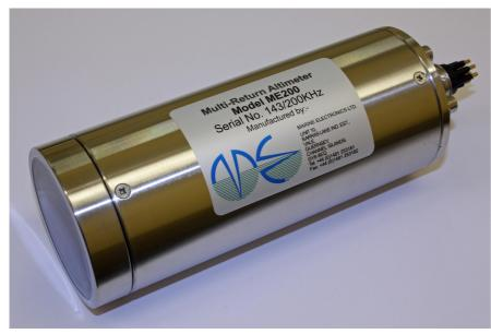
The Model ME200 Altimeter measures the acoustic travel time from the Transducer face to the sea bed and back and is ideally suited for use in water with a high concentration of sediment. For each acoustic pulse the returned echoes are digitised, processed and the range to the seabed transmitted serially via an RS232 or RS485 link, or output as a DC voltage with either +5v or +10v full-scale reading.
