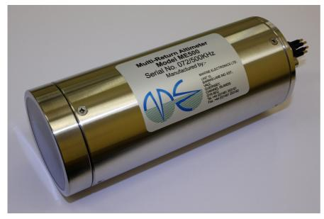
The Model ME500 Altimeter measures acoustic travel time from Transducer face to the sea bed and back and is ideally suited for use in water with a high concentration of sediment. For each acoustic pulse the returned echoes are digitised, processed and the range to the seabed transmitted serially via an RS232 or RS485 link, or output as a DC voltage with either +5v or +10v full-scale reading.
