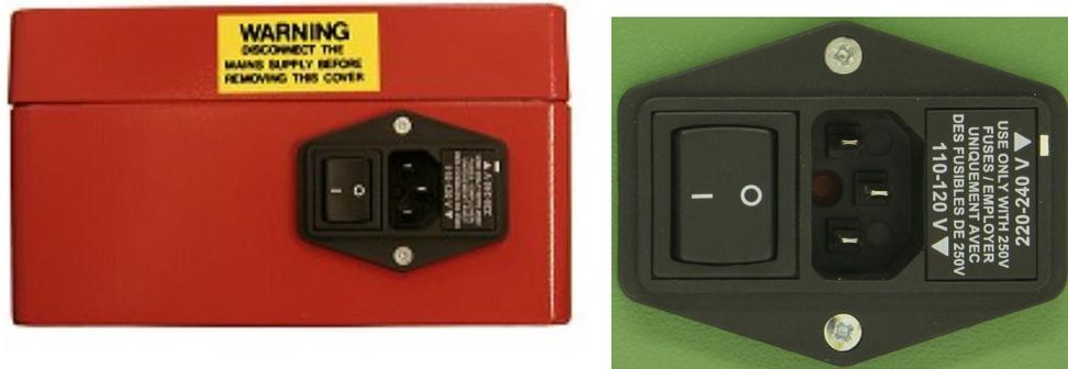
The picture shows the voltage selection set to 240v ac. To change to 110v ac remove the fuse holder and re-insert with the 110v arrow pointing towards the white line.
