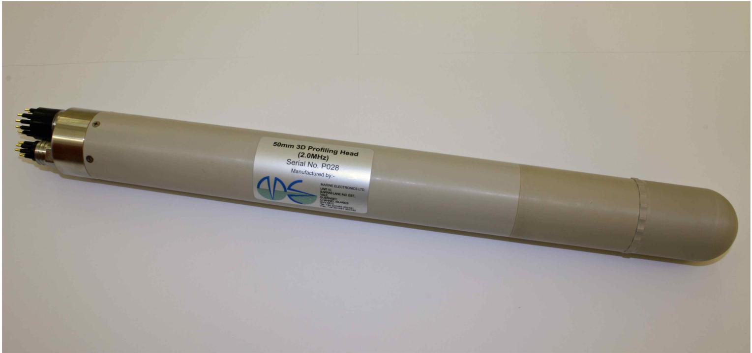
The 3D Profiling Sonar Model 2001-50RH is designed to operate long term in radioactive ponds and settlement tanks and gather high resolution bathymetry data. Manufactured in PEEK and only 50mm in diameter the unit can be installed through the smallest of access points. Multiple units can be linked together and controlled via Ethernet to enable large areas to be fully mapped. The windows software allows images to be merged to produce a single point cloud picture.
