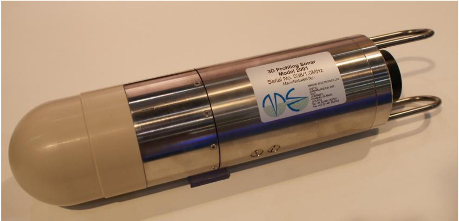
The 3D Profiling Sonar Model 2001-90 is designed to operate long term in enclosed spaces including radioactive ponds and settlement tanks and gather high resolution bathymetry data. Manufactured in PEEK / Stainless Steel and only 90mm in diameter the unit can be installed through the smallest of access points. Multiple units can be linked together and controlled via Ethernet to enable large areas to be fully mapped. The windows software allows images to be merged to produce a single point cloud
