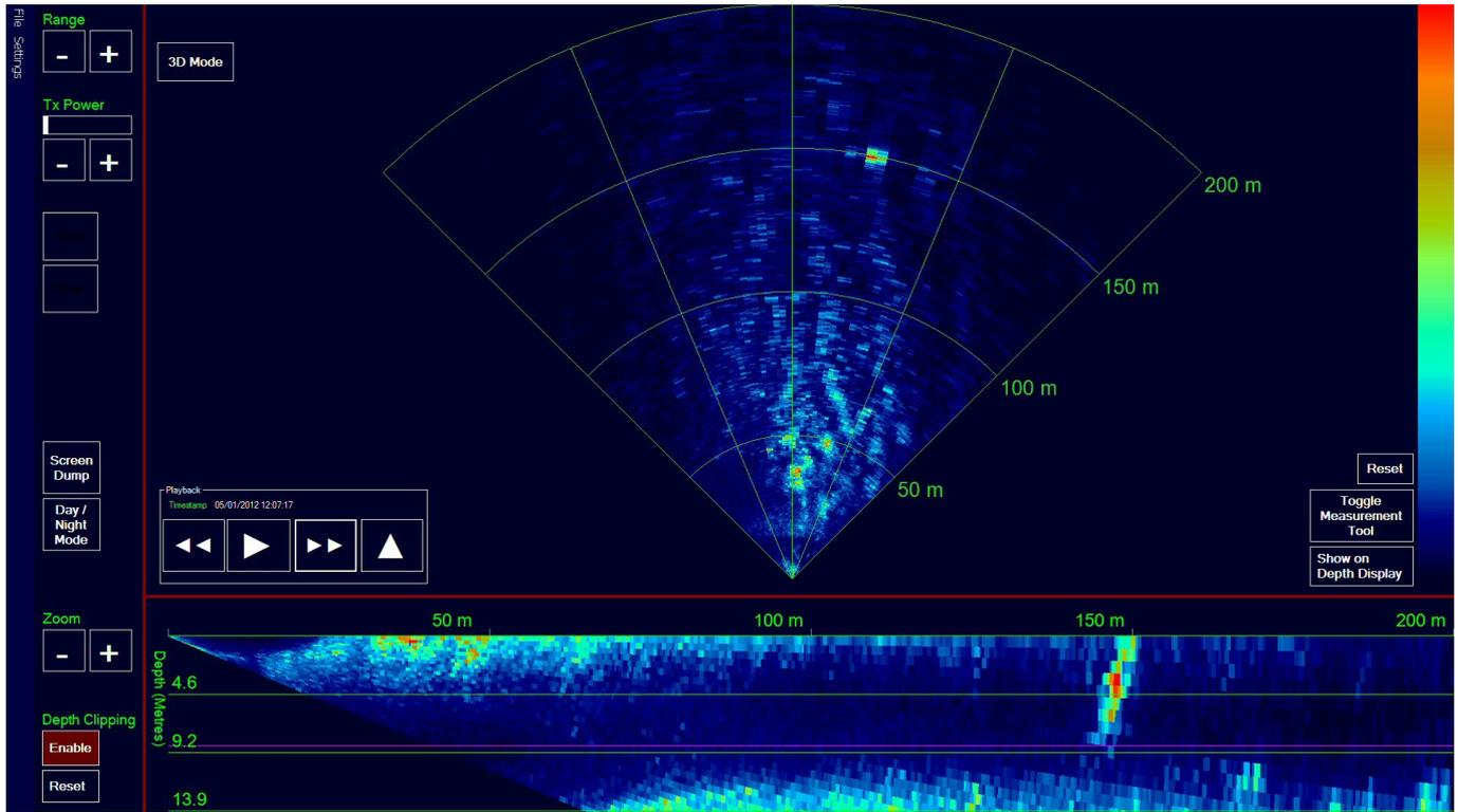
With 3D technology the sonar can discriminate targets anywhere in the water column between the surface and the seabed
