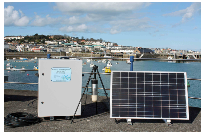
Sonar Head, 4G / Battery Control Box, Solar Panel
