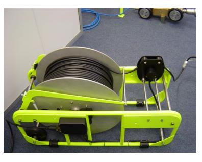
The 300m hand operated cable drum has a slip ring assembly and shaft encoder to monitor the amount of cable deployed. With the handle provided the drum can move easily on its wheels between deployments.
