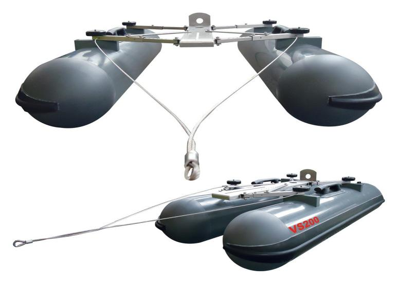
The VS200 Floatation device is designed to carry both Profiling Sonar and CCTV camera for inspection above and below the water line. The float can be adjusted using the arms to operate in a variety of pipes and culverts with a minimum span of 600mm. Fixing eyes either end allow the float to be tethered for free flow or winching. Manufactured from PVC and Stainless Steel and weighing 18.6Kg the float can cater for a maximum payload of 30Kg.
