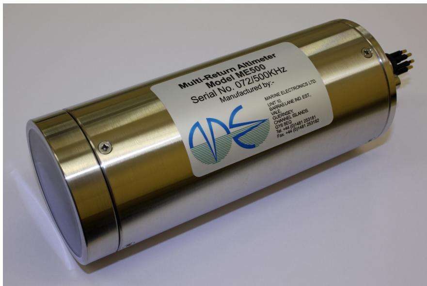
The Model ME500 Altimeter measures the acoustic travel time from the Transducer face to the sea bed and back and is ideally suited for use in water with a high concentration of sediment. For each acoustic pulse the returned echoes are digitised, processed and the range to the seabed transmitted serially via an RS232 or RS485 link, or output as a DC voltage with either +5v or +10v full-scale reading.
