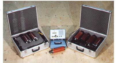
Transponder Control Unit with Remote Active Transducer and 50m cable reel
